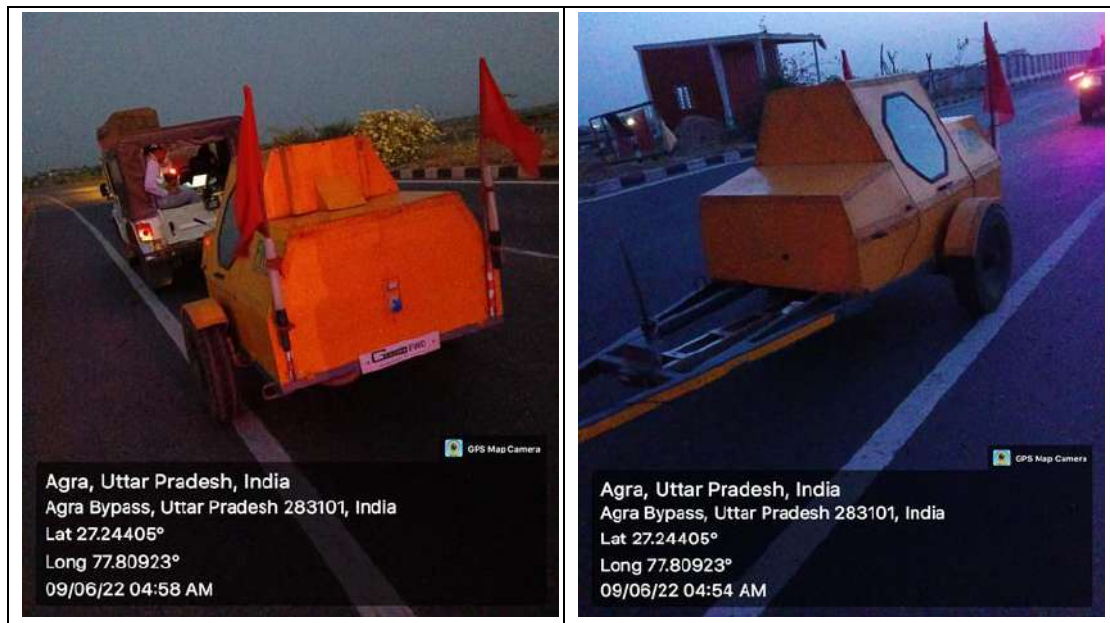
FWD Survey in progress
