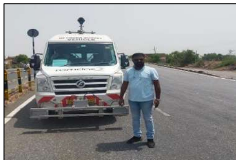
NSV with Laser Profiler
