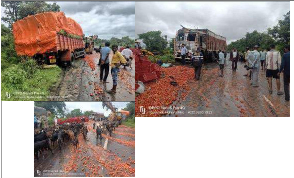
Photo 8: Unbalanced truck accident due to overloading
